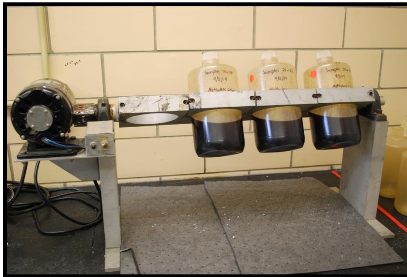
Figure 4.4. HTL samples with methylene chloride solvent being rotated
