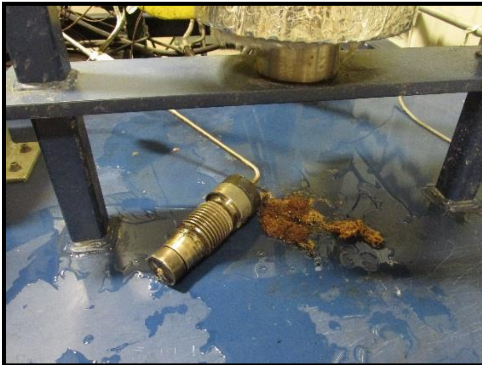
Figure 4.5. Solids that settled out of the SCFR HTL run
