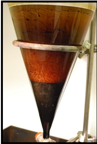
Figure 4.8. Stratification in the separatory funnel of HTL sample aqueous fraction (top layer) and methylene chloride soluble fraction (bottom layer) (left)
